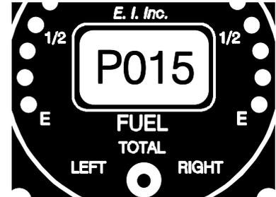
12. To program (change) the fuel level for this calibration point, push and hold the Enter Button on the back of the FL-2 for 3 seconds. The far left letter ("P" or "F") will be blinking. To change this letter, move the selector switch to the left or right.
