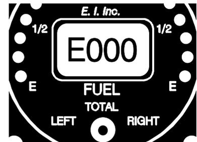
Tap the Enter Button on the back of the FL-2, the display will start blinking and the Sensor Counts for the current fuel level in the tank will be displayed. Wait for the display to stabilize and tap the Enter Button to lock the current Sensor Counts into the display and stop the blinking.
