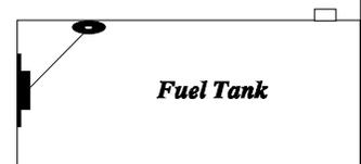
3. As you raise the sensor float **slightly** off the bottom of the tank, the resistance should start to increase. If it does not, the sensor resistance is probably bottomed out. The FL-2 will read lower than actual fuel levels until the sensor wiper drops onto the resistive element.
