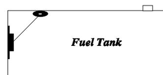
With the sensor float held to the bottom of the tank, adjust the sensor float arm so the wiper is on the resistive element and not on the termination (end stop). You will need an ohmmeter to determine this. As you slightly move the float arm, the resistance should change.
