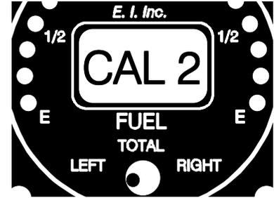
10. Fill the tank to the fuel level indicated on your calibration chart for the next calibration point.
