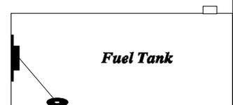
2. With the float at the top of the tank (as it would be if the tank was full), measure the resistance of the fuel sensor. The resistance should be between 270 ohms and 90 ohms. If the readings are below 90 ohms or greater than 270 ohms, you may be using the wrong type of sensor. Use a sensor that increases resistance when fuel is added and has a maximum resistance of between 90 and 270 ohms.
