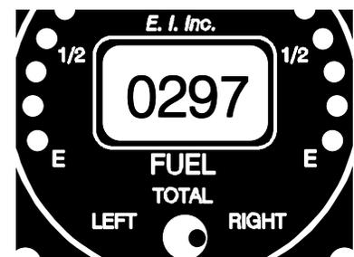
Note: If you want to manually program the Sensor Counts, push and hold the Enter Button at the back of the FL-2 (with the Sensor Counts displayed and not blinking) until the thousands digits starts to blink.
