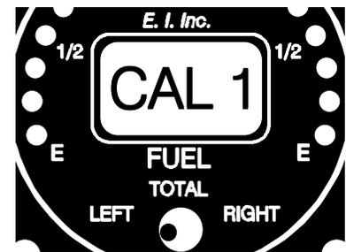
Note: If you are recalibrating the FL-2 and wanted to advance to a specific calibration point, push and hold the Enter Button on the back of the FL-2 until you get to the calibration point of interest. The calibration points will advance every 3 seconds. If you accidentally advance past the full fuel calibration point, the FL-2 will check for errors, go through the power-up sequence and then into the normal operating mode. You will have to start over.
