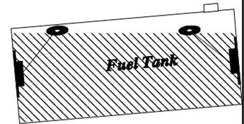
Fuel slosh to the in-board or out-board portion of the tank can also cause inaccurate readings. For example: depending on the fuel sensor placement in the tank, as the fuel sloshes to the out-board portion of the tank during a turn, the fuel level reading on an in-board mounted sensor will lower,
