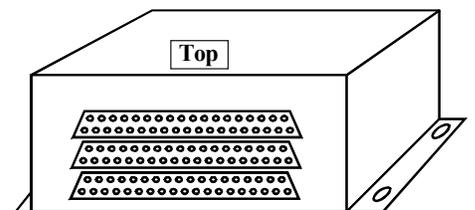
When routing the EDC wire harnesses refer to the Top, Middle and Bottom "EDC Wiring Work Sheets" found at the back of this manual. Insure no wires obstruct the freedom of travel of any controls.
