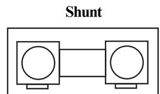
The signal wires from the shunt to the EDC must be fused a short distance after they leave the shunt. If this is a new installation, install two in-line one-amp fuses, one in each of the signal lines from the shunt to the EDC Amp Input.
