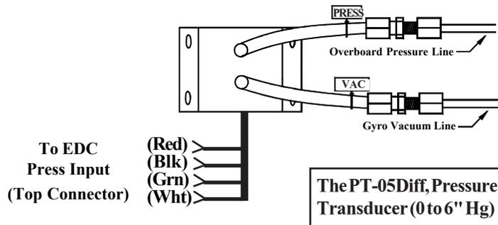
Connect the aircraft gyro vacuum line to the port tagged "Vac" on the PT-05Diff. Connect the port tagged "Press" to the aircraft overboard pressure line. A flare or barb fitting may be used to connect these lines. Care should be taken not to put excess pressure on the flexible line leading to the pressure transducer. **Make sure there are no kinks in the flexible pressure lines.**
