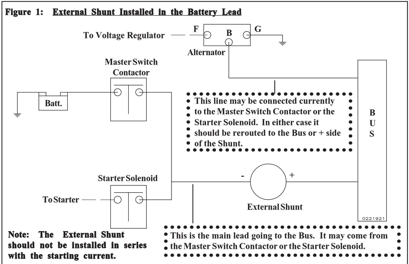
**Note:** If you are replacing an existing ammeter, the shunt may already be mounted in the aircraft. If you already have a shunt installed and know the value of the existing shunt, the CGR can be calibrated to that shunt.
