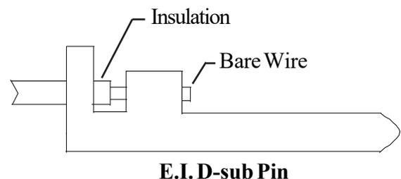
C. Insert the wire into the pin. Check that the insulation is in the strain relief crimp area but not in the bare wire crimp area. Crimp the pin onto the wire. **A good crimp is very important. Poor crimps will cause jumpy readings and are the biggest source of problems.**
