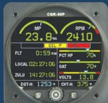
The secondary screen, above, announces main page alerts while displaying six additional engine monitoring functions.
