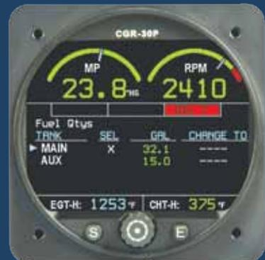
The fuel quantity screen displays the estimated fuel remaining for each tank, above.
