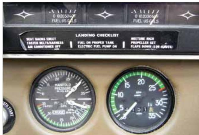
*The CGR-30P display, left, is designed as a replacement for the mechanical tachometer, manifold pressure and fuel gauges, above. While these factory gauges are often placed in the lower sub-panel, your shop might need to find an alternate location that's in your direct field of view.*
